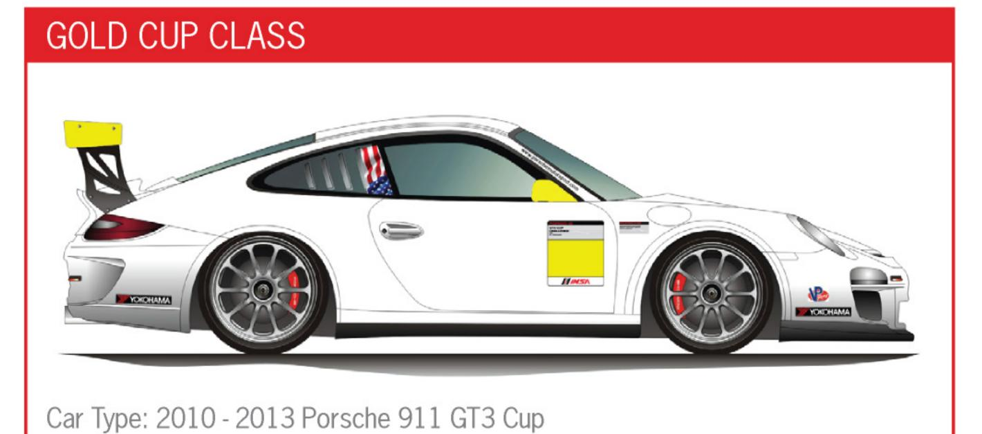
Engine: 3.8L, 6-cylinder naturally aspirated | Produces: 450 bhp at 8500 rpm
